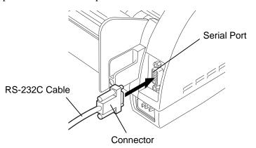
**3.** Secure the connector with the screws.
